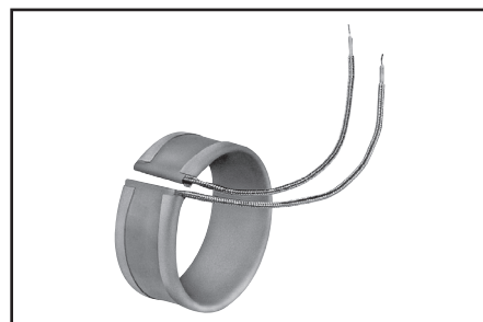
Fig. 3 – Single conductor metal braid over lead wire. Offers most practical solution to abrasion problem. 12" braid with 14" overall length leads are standard.
