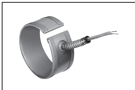
Fig. 6 – Flexible armor cable is the best solution to lead abrasion problems. 12" armor with 14" overall length leads are standard. Specify alternate position.
